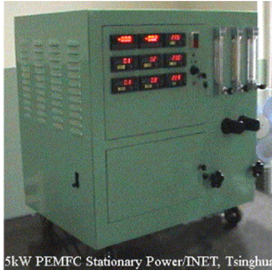
Fig. 6. Appearance of the 5 kW PEMFC stationary power system [61].
