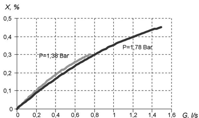
Fig. 6. Inversion point dependence on gas flow in spiral wound membrane contactor.
