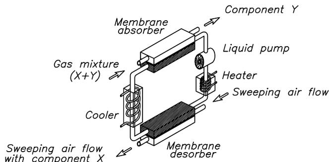
Fig. 4. Recycle membrane contactor.
