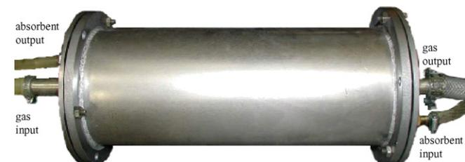
Fig. 2. Spiral wound membrane module.
