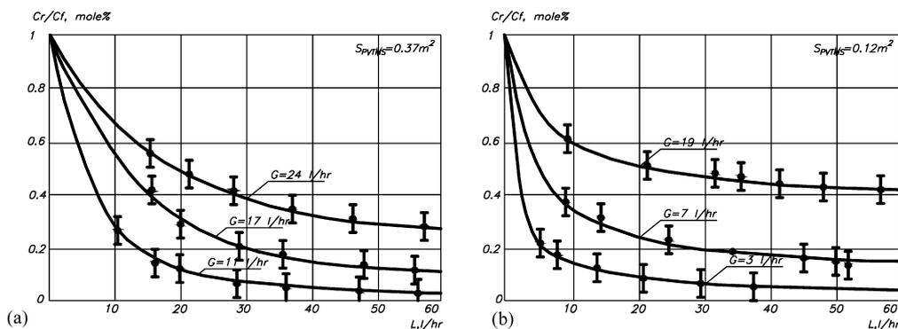
Fig. 8. Relative CO<sub>2</sub> concentration dependence on liquid absorbent flow for flat frame membrane contactor: (a)  $S_{PVTMS} = 0.37 \text{ m}^2$  and (b)  $S_{PVTMS} = 0.12 \text{ m}^2$ .
