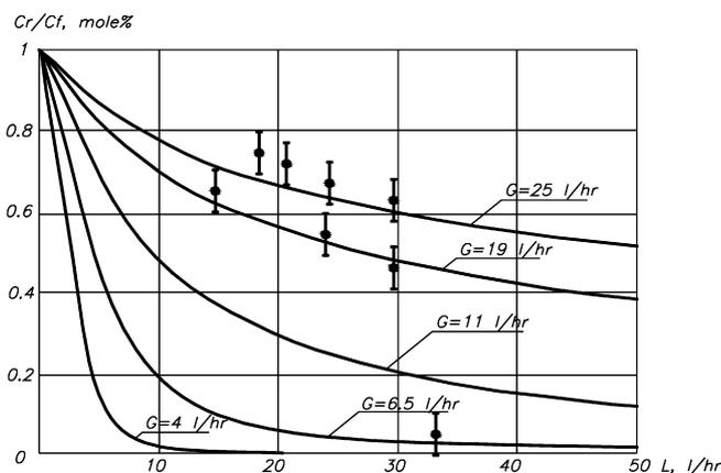
Fig. 7. Relative CO<sub>2</sub> concentration dependence on liquid absorbent flow for spiral wound membrane contactor.
