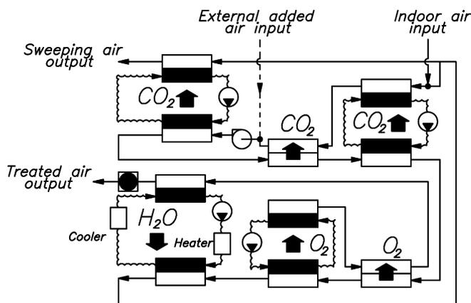
Fig. 1. Recycle membrane contactor (RMC) air conditioning system principle.
