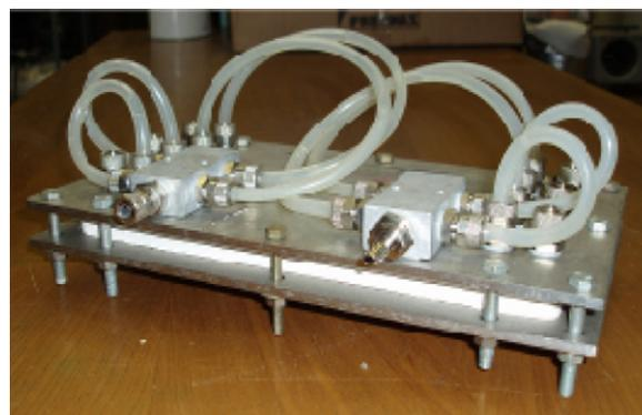
Fig. 3. Pilot flat frame membrane module.
