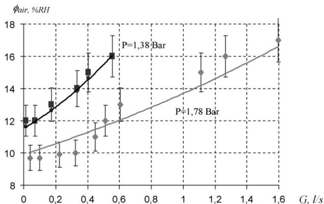
Fig. 5. Air humidity dependence on feed gas flow in spiral wound membrane contactor.
