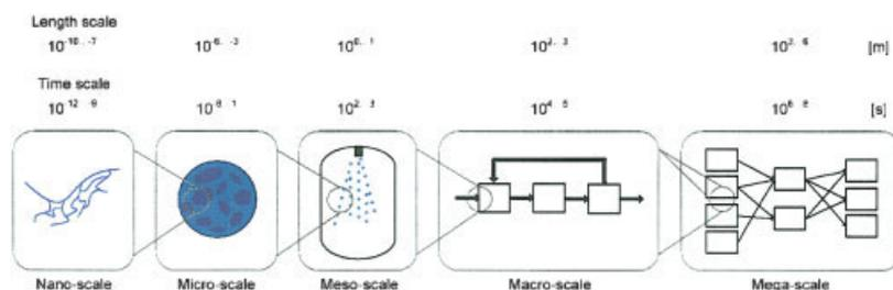
Figure 6. Length and time scales in the development of a powdered detergent (adapted from Edwards<sup>51</sup>).
