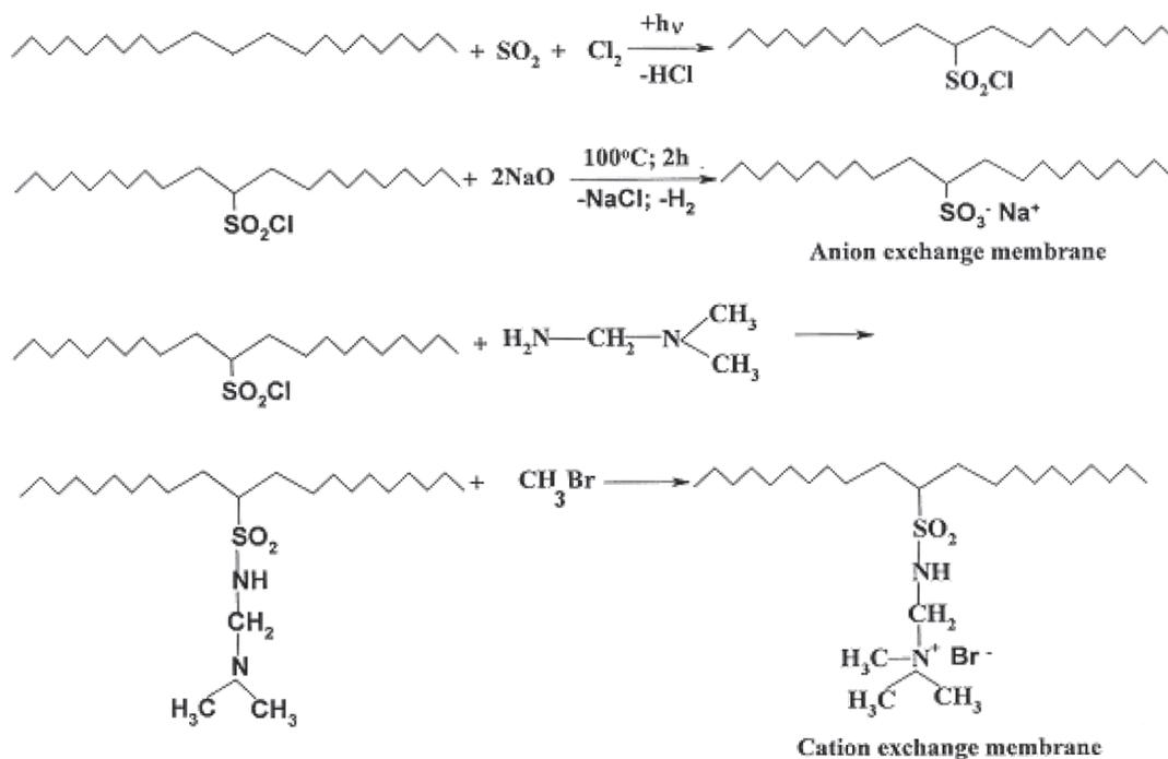
Fig. 11. Schematic presentation of grafting of polyethylene membrane.
