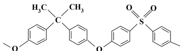
Fig. 7. Structure of Udel polysulfone.
