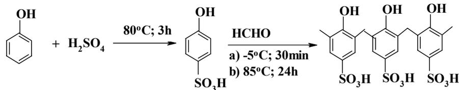
Fig. 1. Reaction of phenol sulfonic acid with formaldehyde.
